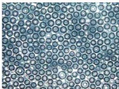
FIG. 3 (color online). Air bubbles in the liquid crystal matrix. The width of the image is 1.75 mm.
