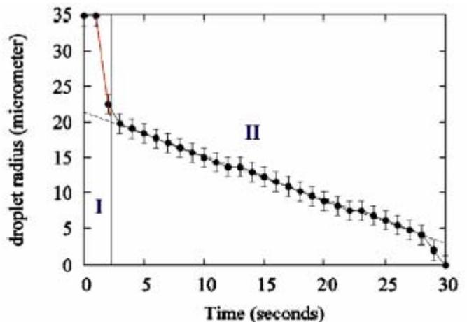
FIG. 6 (color online). Two distinct regions of the shrinking of the air bubble: Compression of the bubble by high pressure (region I) and shrinking of the bubble due to the absorption of the air into the liquid crystal (region II). The external pressure made a jump from 100 to 500 kPa in region I and was kept constant throughout region II.
