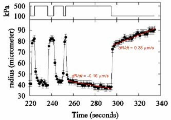
FIG. 5 (color online). Change of bubble radius (bottom graph) by applying and releasing high pressure (change between 100 and 500 kPa, top graph).
