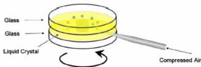
FIG. 2 (color online). Experimental setup: Gas bubbles are injected through a capillary into the liquid crystal which is contained in a rotating sandwich cell.
