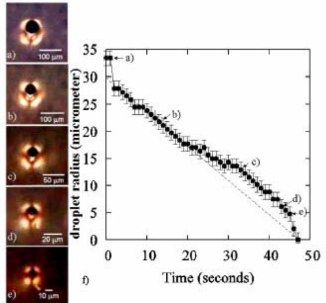
FIG. 7 (color online). (a)–(e) Inducing a transition from a dipolar hyperbolic hedgehog configuration [(a)–(d)] to a quadrupolar Saturn-ring configuration [(e)] by decreasing the radius of the gas inclusion. 500 kPa (initial pressure 100 kPa) is applied in order to induce the shrinking of the bubble size. (f) Bubble radius as a function of time.
