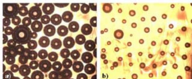
FIG. 4 (color online). Control of bubble size using the pressure technique. Gas bubbles at (a) 100 and (b) 640 kPa. The width of the images is 1.57 mm.
