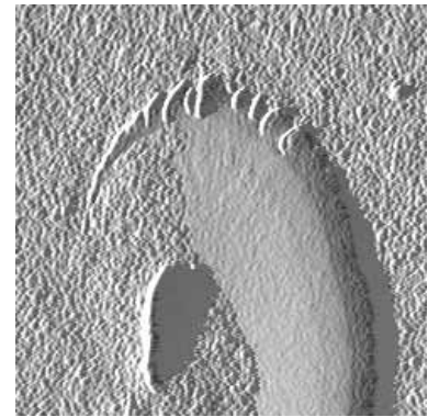
Fig. 4 AFM images of a PE single crystal grown from the melt. 1.6 \times 1.6 \mu\text{m}^2
