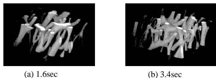
Fig. 2. Morphological change under shear flow and electric field after applying an electric field of 2 kV/mm.
