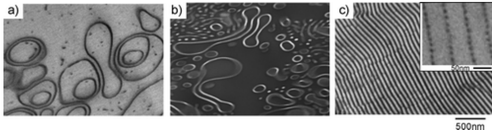
Figure 1. Bright Field TEM images for SH/IP 5:5 blend films from THF ((a) and (b)), and THF/toluene(c). Sample specimens were stained with OsO 4 .
